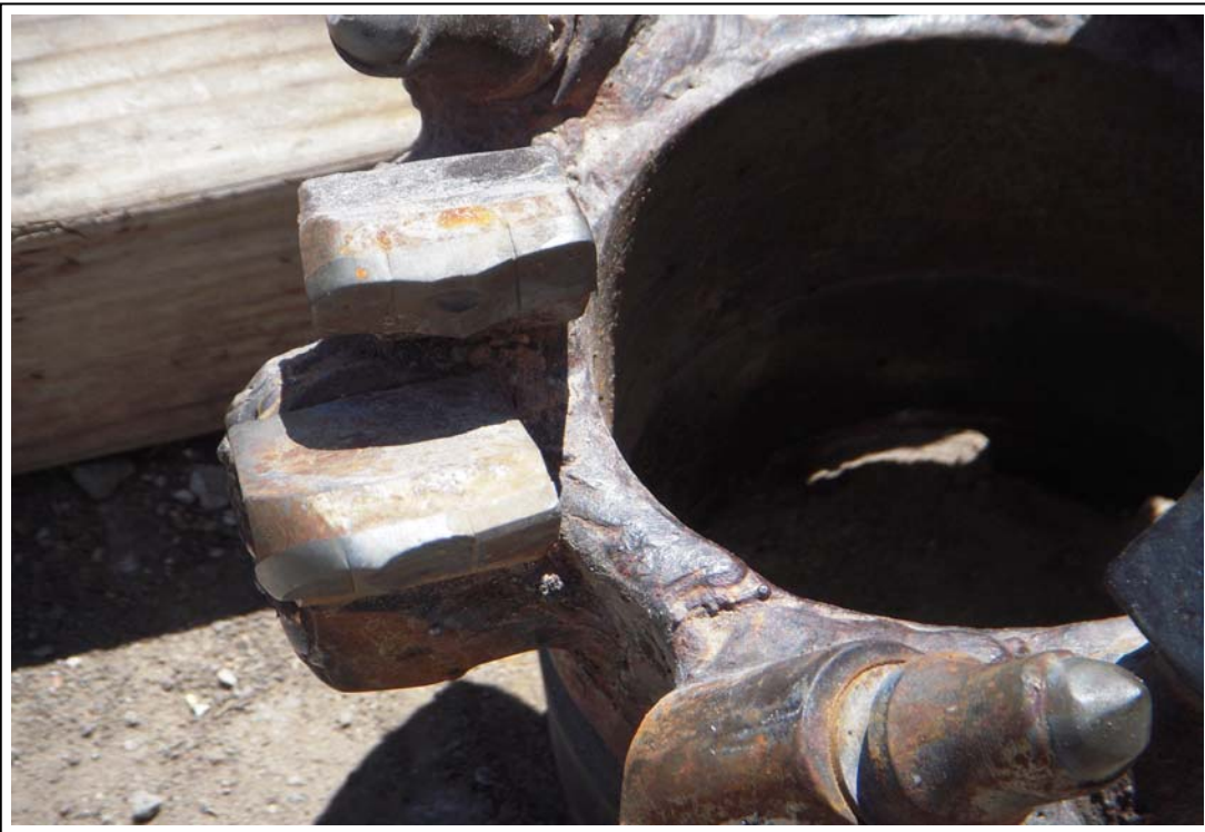
8. Auger bit with flat and bullet teeth that both contain lead with highest concentration in the tips of the teeth (tungsten carbide tips are not rusted).
