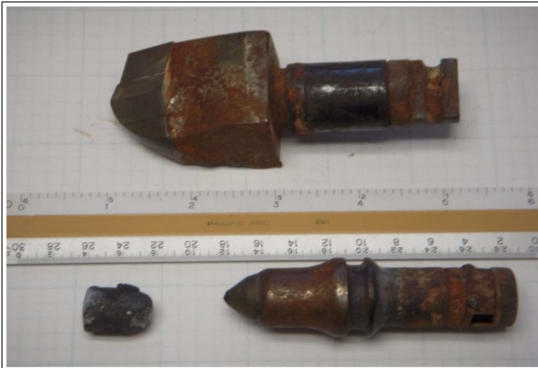
9. Three drill bits collected for this study. Top = HSA flat bit; bottom left = tricone bit, bottom right = HSA round bit.
