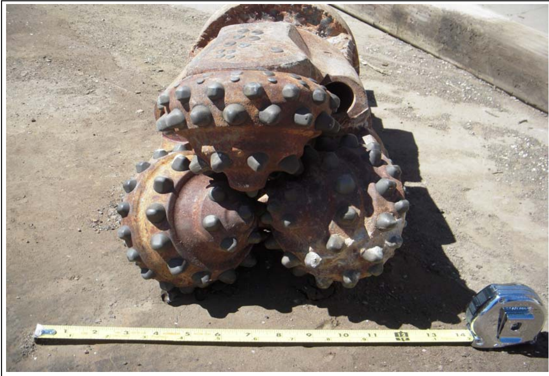
9. Tri-cone bit with gray teeth containing lead
